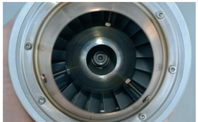
It is difficult to get a good photo inside the tailcone, but the turbine wheel and internal fairing can be seen here
