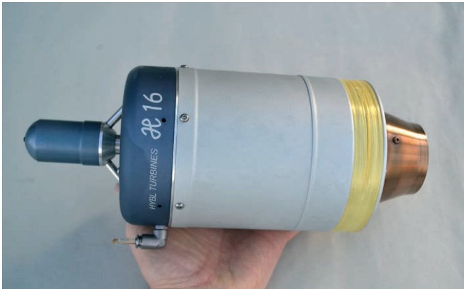
The H16 has a very clean external appearance, with the thermocouple and kerostart igniter being internally installed
