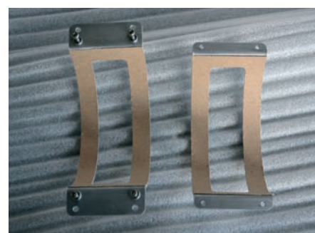
The manual suggested fitting thick paper to the engine mounts to avoid marking the outer surface of the turbine; so heavy brown paper was used during testing
