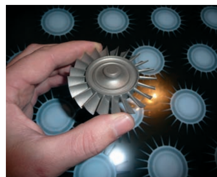
A close-up of the cast turbine wheel, with a sheet of X-Rays of each turbine wheel in the background
