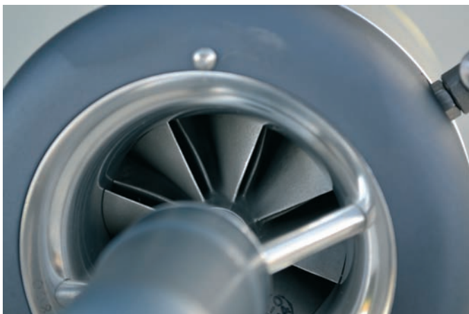
Very precise casting work is evident on the compressor blades
